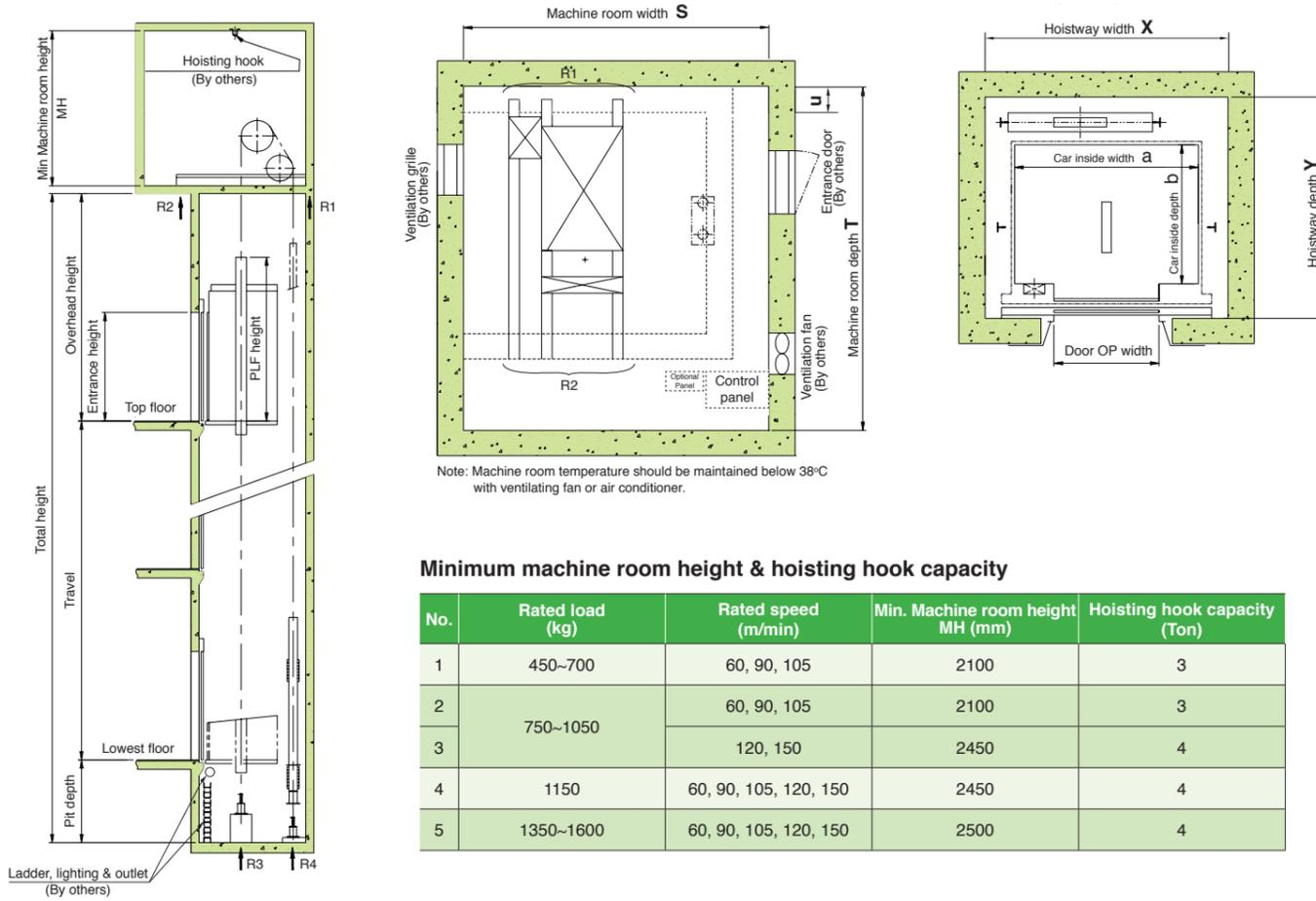
**Minimum machine room height & hoisting hook capacity**
