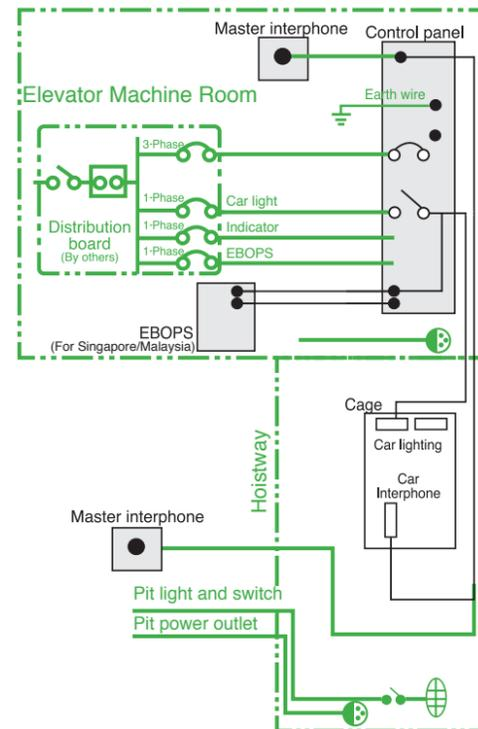
(\*) Main and lighting supply shall lead into the elevator machine room.
